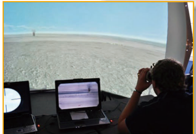
VSS Dome Screen used with VSS VR binoculars in Forward Observer/JTAC simulation
